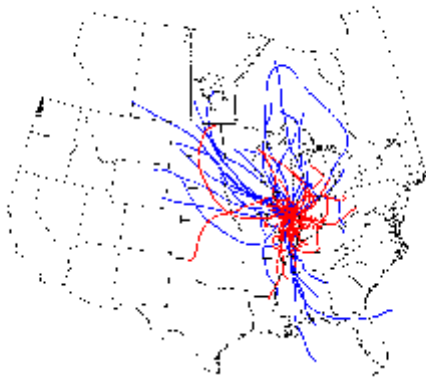
48-Hour Backward Trajectories for Bondville CYSINCT Site Site Height = 500 m. Red Days: n = 5, Blue Days: n = 5.
