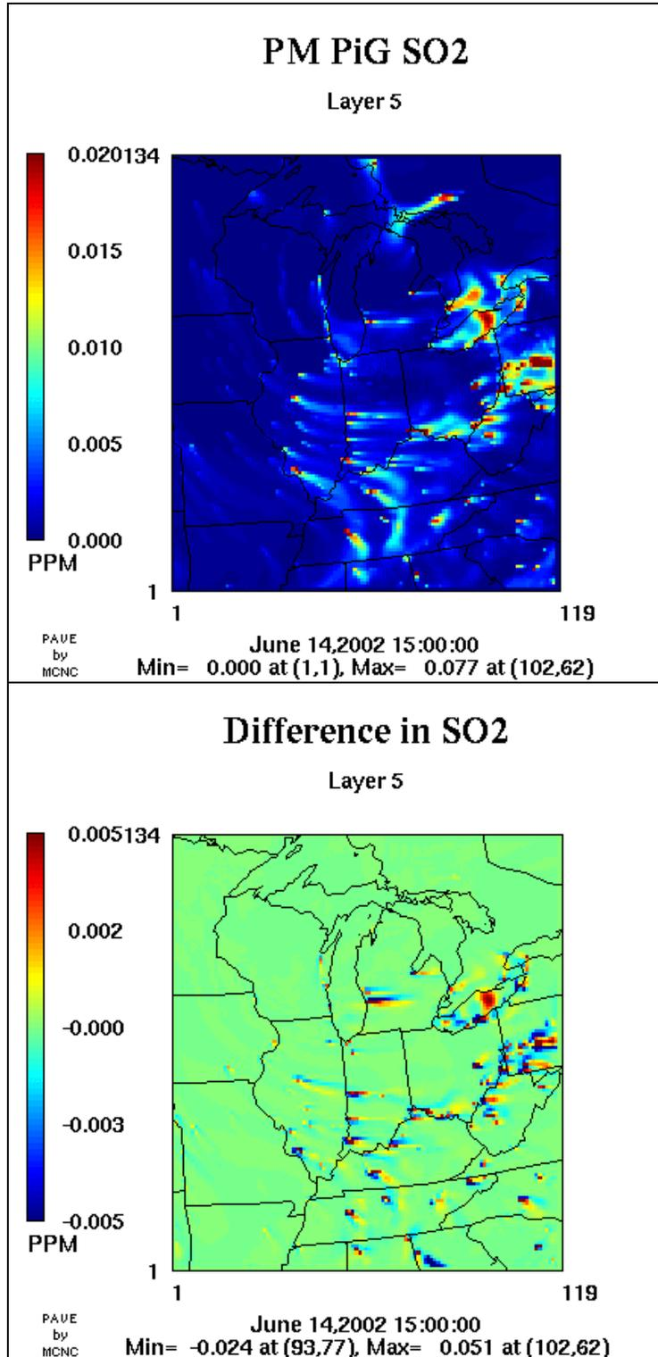
**Figure 4-3.** SO<sub>2</sub> concentrations (ppm) in layer 5 for the PM PiG run (top) and for the difference between the PM PiG and no-PiG runs (bottom).
