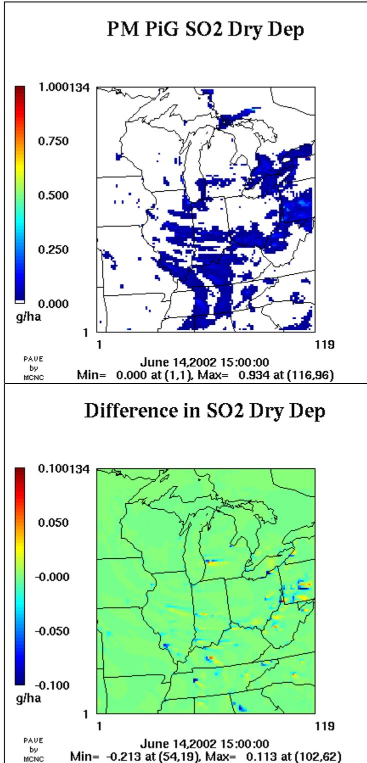
**Figure 4-9.** SO<sub>2</sub> dry deposited mass (g/ha) for the PM PiG run (top) and for the difference between the PM PiG and no-PiG runs (bottom).
