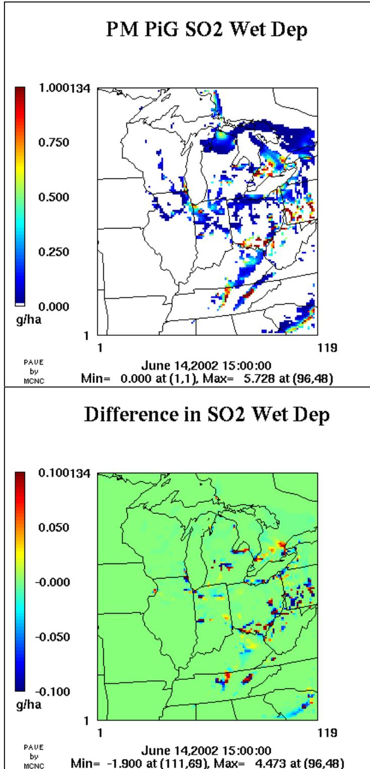
**Figure 4-10.** SO<sub>2</sub> wet deposited mass (g/ha) for the PM PiG run (top) and for the difference between the PM PiG and no-PiG runs (bottom).
