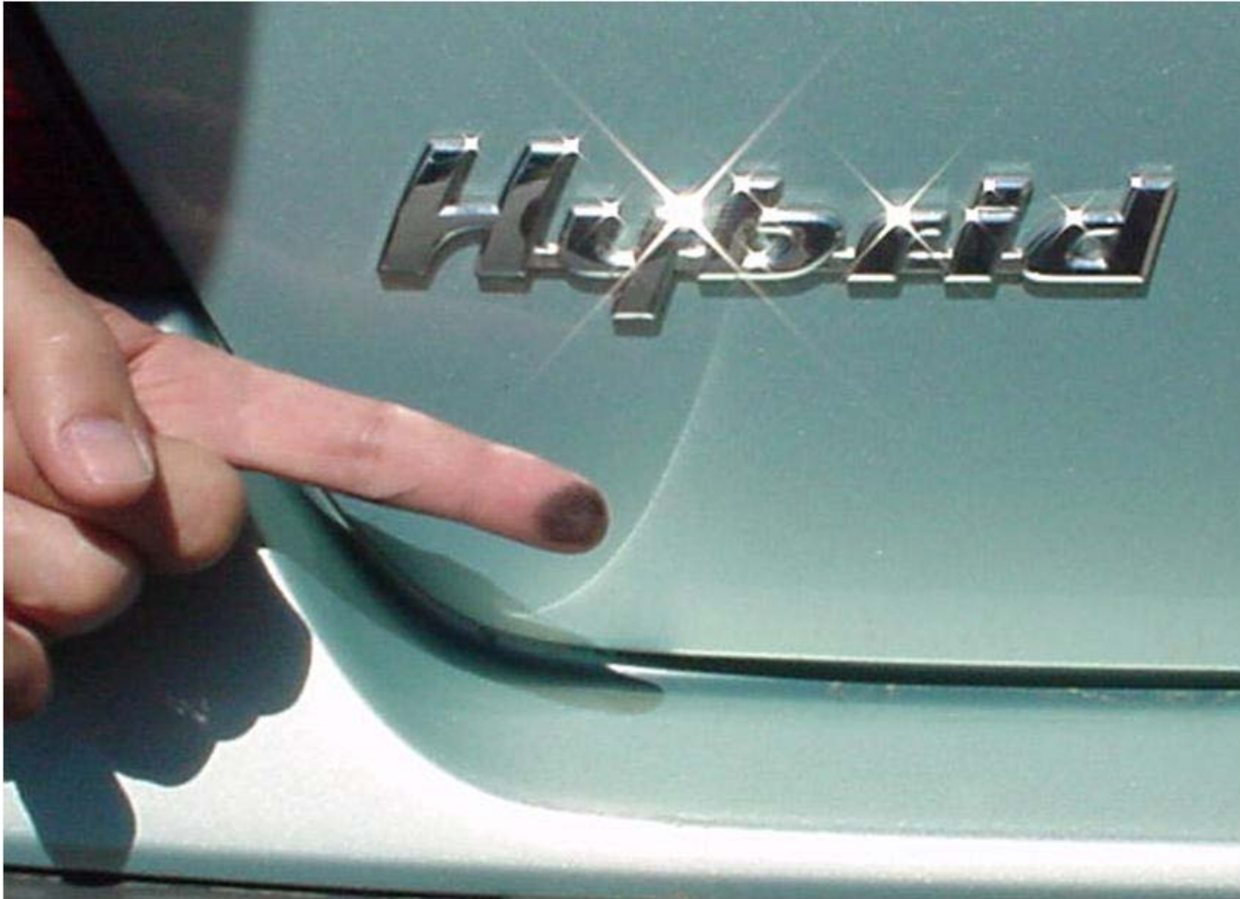
Soot from the tailpipe of a low-mileage Prius at NREL
